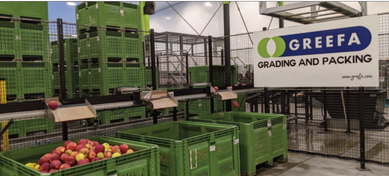
The Greefa pre-sorting line can handle 12,000 kilograms of apples per hour, taking bins out of controlled atmosphere storage, scanning and tracing each bin as they move down the line.
