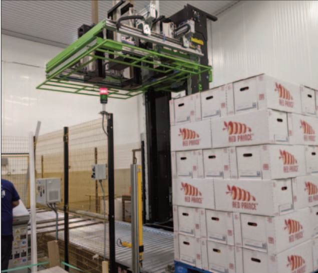
The palletizer is a labour-saving device in a complex operation of moving apples to their final destination.
