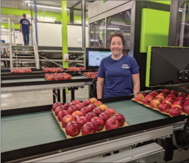
Sacha Botden supervises the tray line. It consists of four automatic tray packers which can handle up to 170 apples per minute.
