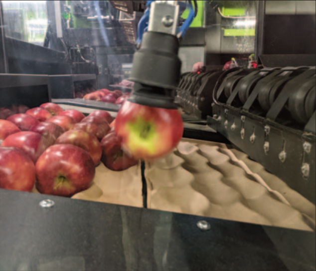
The robotic arm makes sure that each apple is settled gently into its nesting cavity.
